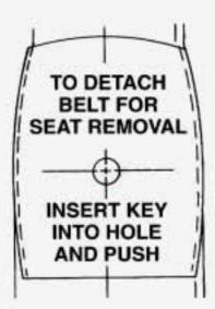
If you are removing the center seat, remove the right lap—shoulder belt. To do this, press the tip of a key into the release hole of the safety belt attachment while pulling up on the safety belt.
